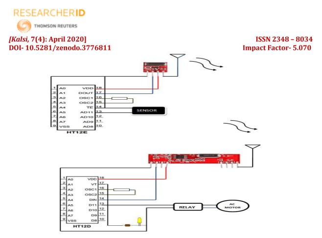
Figure 6: Circuit Diagram of the project
