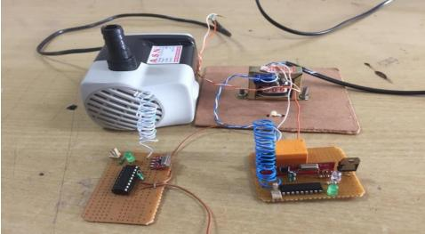
Figure 7: Implementation of the water detection system
