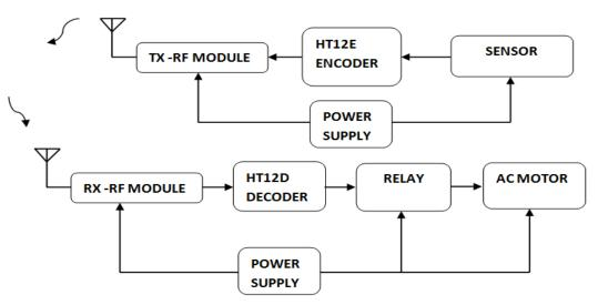
Figure 3: Block Diagram of automated water level controller
